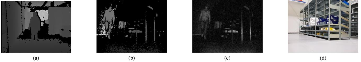
Fig. 2. Comparison between (a) BIWI depth image and (b) PicoFlexx IR gray value image created from (c) PicoFlexx point cloud. The BIWI depth image has an increased brightness for a better representation. In (d) is the scene from (b) and (c) captured as RGB-image, for logistic context in front of shelves.
