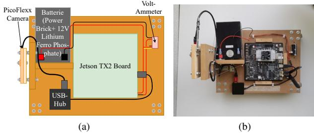
Fig. 3. Experimental bare-bone setup, as sketch in (a) and assembled in (b).
