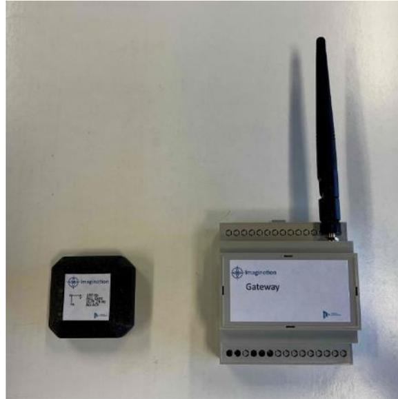
Figure 16. Imagination measurement set - sensor and DIN-rail mounted gateway with possibility to trigger measurement with digital signal.
