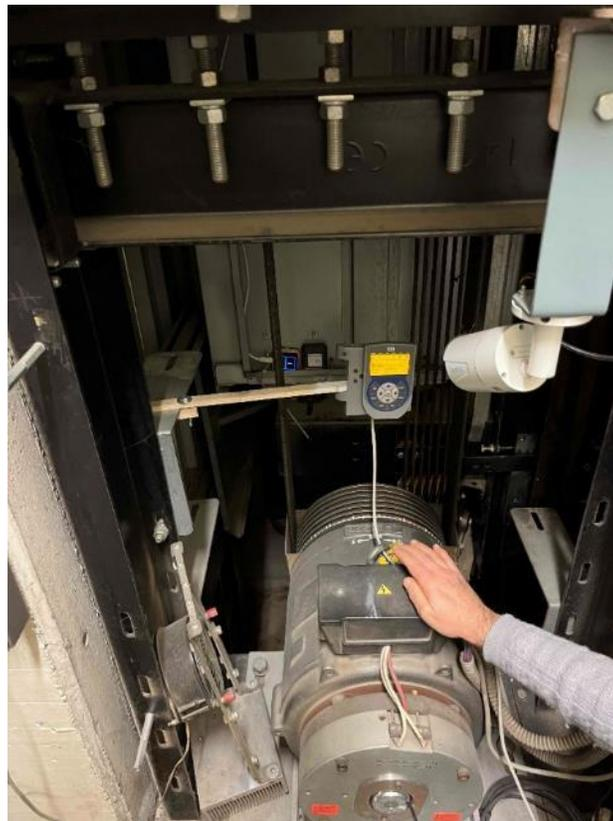
Figure 17. Imagination sensor mounted on a lift cabin in test shaft in WEG. Our sensor (black) is mounted next to the commercial reference sensor (orange/black).
