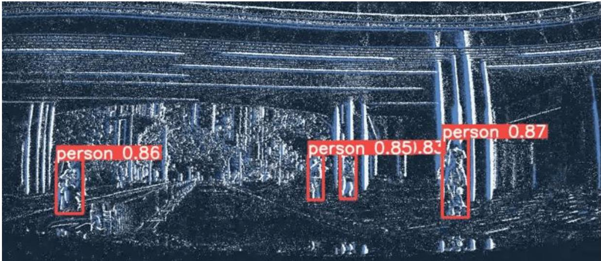
Figure 49. Visualized results of human detection, numbers represent confidence values.
