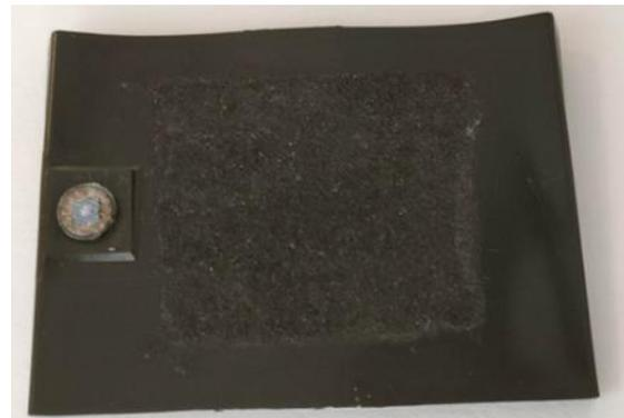
d) Plastic component with sample overmoulded after the ejection.
