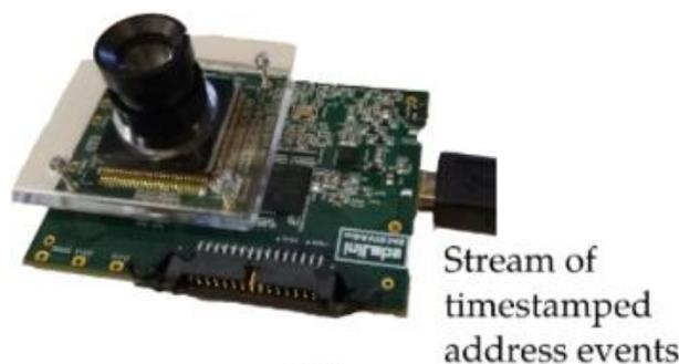
Figure 46. DVS USB camera.
