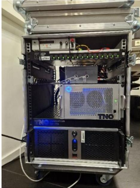
*Figure 117. Computer rack with host PC, PCI-extender, Main switch units and auxiliary electronics box*
