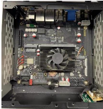
Figure 48. RK3588 computing board.
