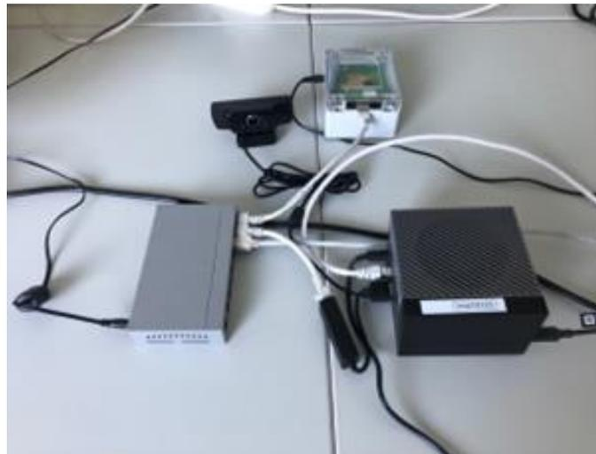
Figure 67. Assembly of Jetson-PC and connected sensors via Ethernet switch.
