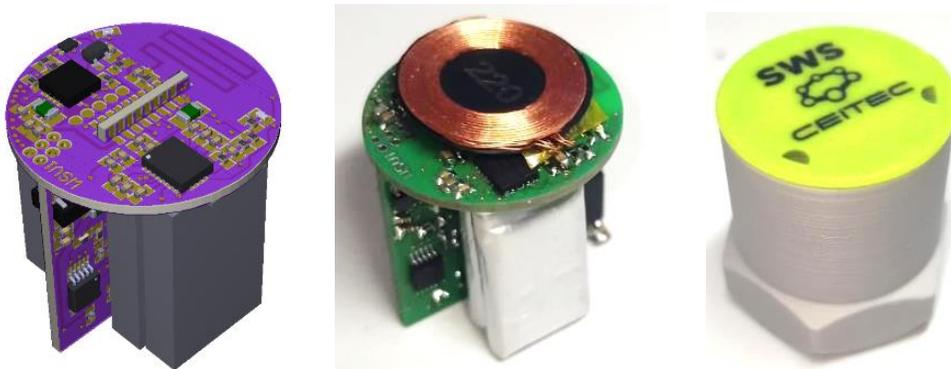
Figure 6. Render of the PCBs (left), real prototype of the assembled sensor (middle) and sensor encapsulated in the 3D printed housing (right).
