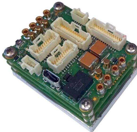
Figure 152. AMC servo drive.
