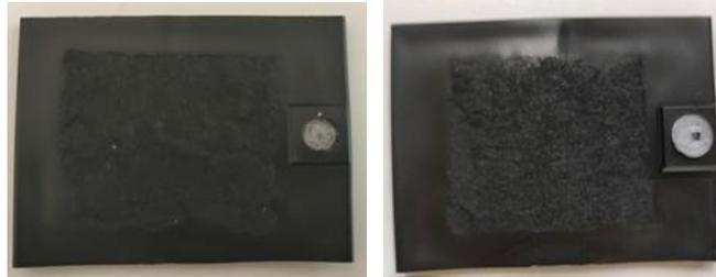
Figure 32. Injection molded part with overmolded encapsulated sensor.
