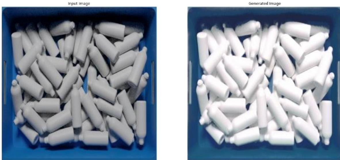
Figure 107. Sim2Real translation example. Synthetic image on the left is made more lifelike and displayed on the right side.
