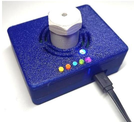
Figure 4. Photography of the designed wireless gateway.
