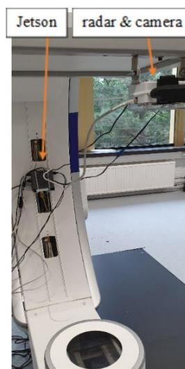
Figure 70. Radar, Camera are connected over the Jetson PC on a Philipps C-arc.
