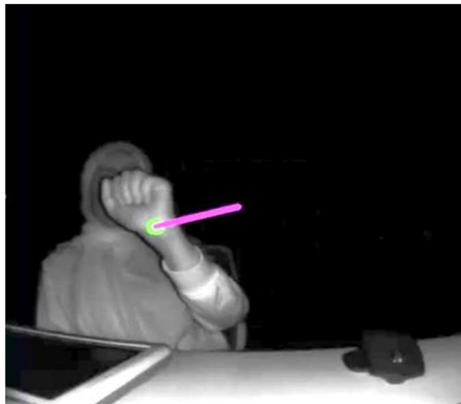
Figure 37. ADF3175 ToF Wrist Tracking in UC3.
