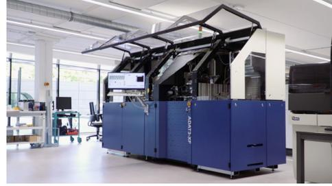
Fig. 1. ITEC's ADAT3-XF die bonder platform. [11]
